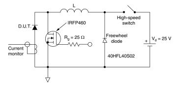
Fig. 7 - Unclamped Inductive Test Circuit
